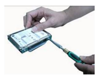
Step 6 Install and fix the HDD through the bottom & side, next, plug the power cable in HDD.
